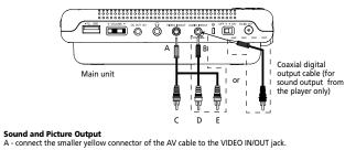
onnect the black connector of the AV cable to the AUDIO IN/OUT jack. Alternatively, connect the ler connector of the coaxial digital output cable (included) for better sound quality.
